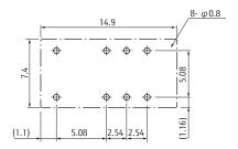
NAL-D (double winding latching type)
